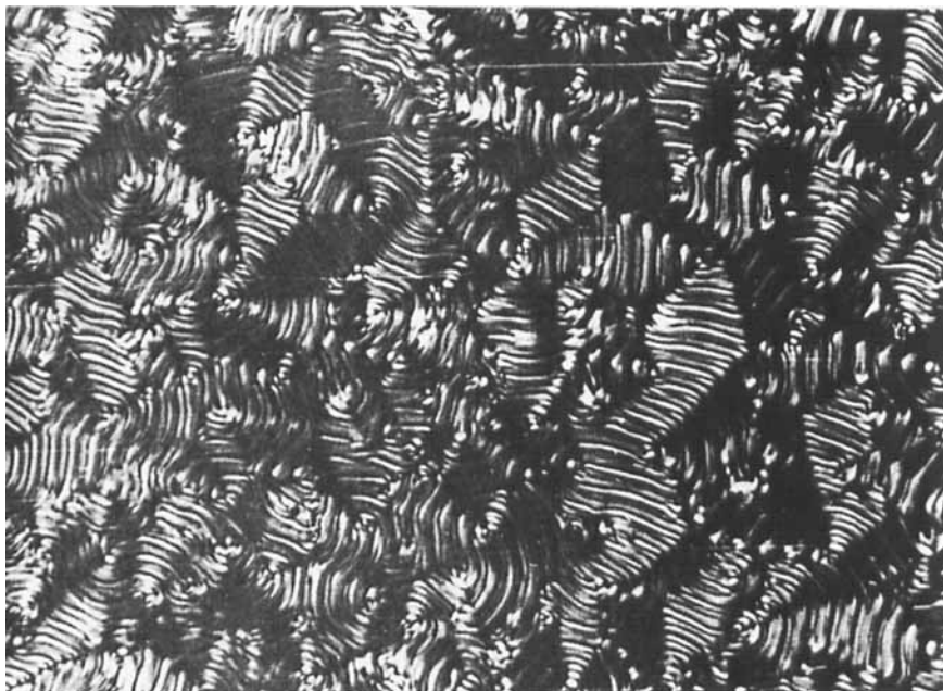
FIGURE 2g Texture of the CC-CP mixture at E = 0.7 E_{CN} ; t = 55^{\circ}\text{C} ; 300\times .
