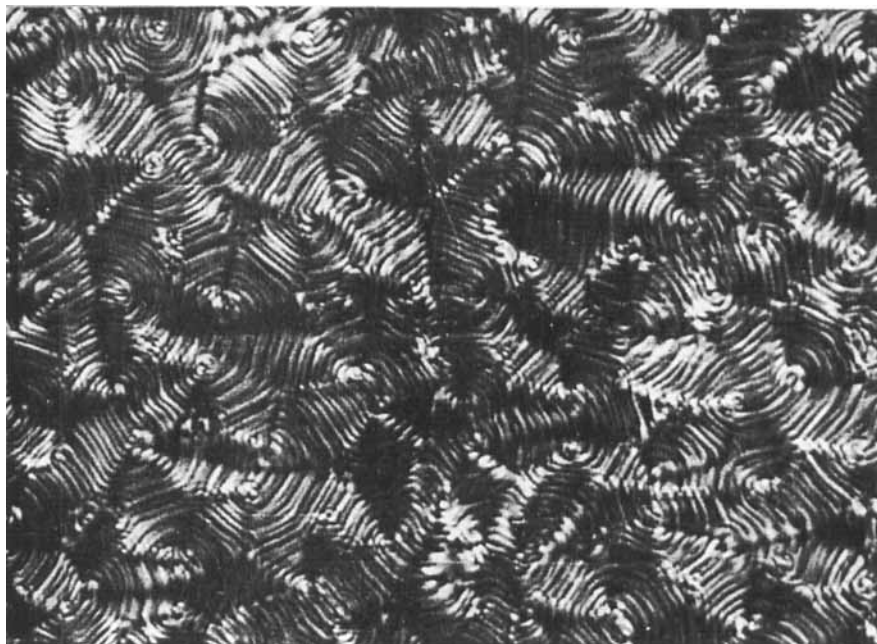
FIGURE 2d Texture of CC-CP mixture, corresponding to the Figure 2c; 300\times .
