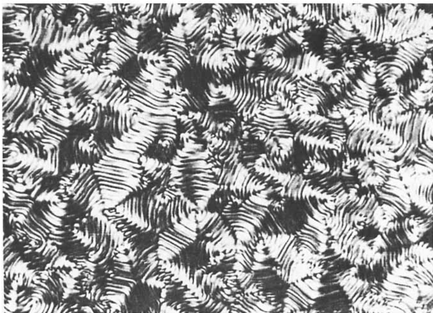
FIGURE 2h Texture of Figure 2g after 30 sec. as the field had been turned off; P —maximum in light scattering pattern disappeared.
